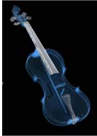
Top: This CT image shows a “sagittal” view of a rare violin. Left: This transparent view of a violin box came from adjusting volume rendering parameters, allowing for an “inside” look at the violin’s sound post and bass bar.
