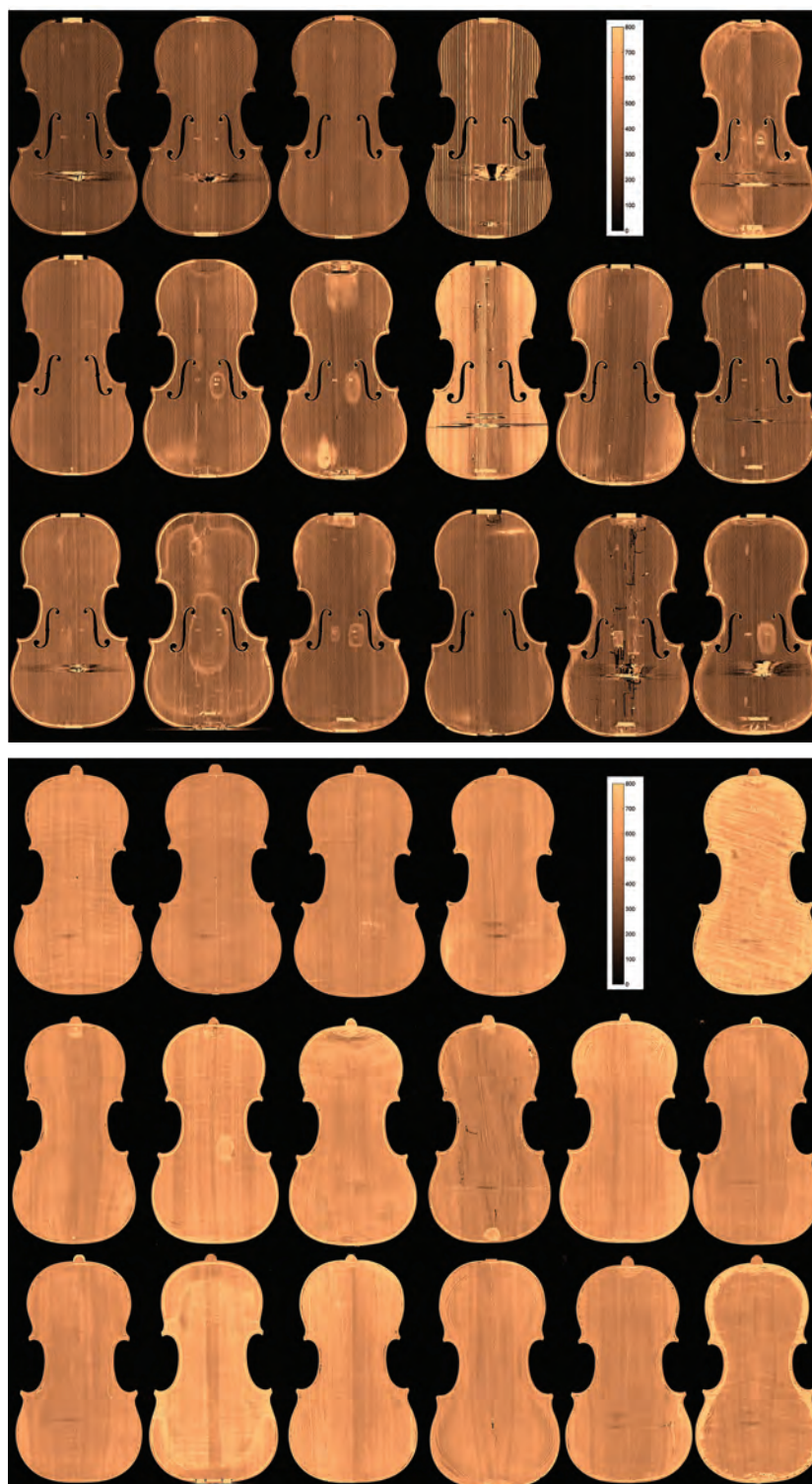
▲ FIGURES 2 and 3 Density maps were made for each of the 17 instruments scanned (top and back)
